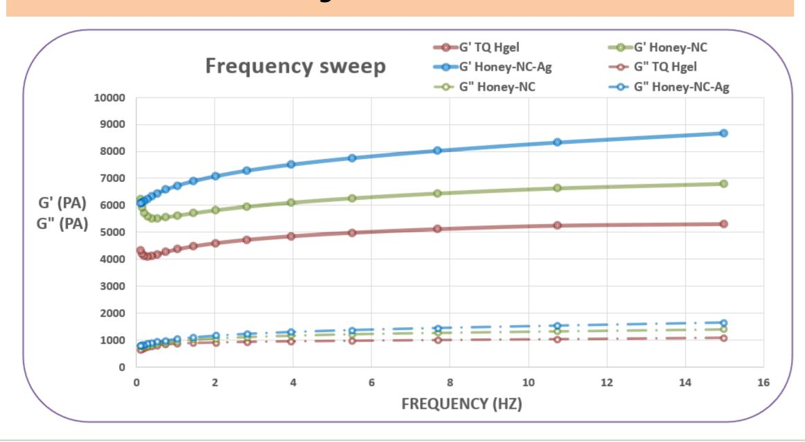
The presence of honey and NC affects the viscoelastic behavior of the hydrogels. These results suggested that incorporating them with AgNPs inside the matrix increase the mechanical strength in both G' and G" compared with TQ hydrogel.
