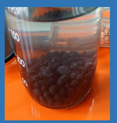
For the treatment of contaminated water, nanotraps were also designed and tested by immobilizing magnetic nanoparticles within biopolymer spheres. This configuration allows for easy recovery of the nanoparticles after treatment, while maintaining high adsorption performance and environmental compatibility.
