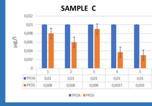
I PFAS adsorbed with the magnetic nanoparticles inserted into the cartridges were first desorbed and then analyzed by UHPLC-MS/MS. (samples A, B, C)
